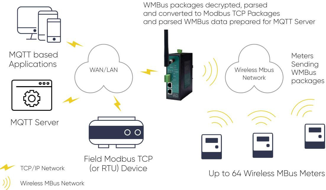
STG In all function modes 1-2-3-4-5-6: STG can decrypt up to 64 devices frames, for example in Function 6: Repeater function.
