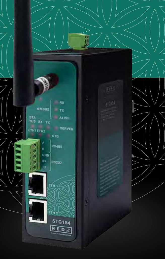
STG Series WMBus Gateways can get Wireless MBus frames over air, Decrypt Up to 64 device packets, parse and map those parsed data to Modbus registers as well as send data to MQTT Server. STG has auto configuration feature to automatically list the received WMBus packages on configuration web interface for easy configuration. STG has 6 Device Functions:
